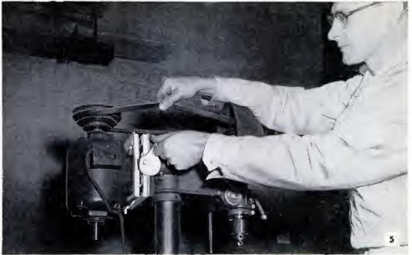
5. HINGED MOTOR MOUNT provides easy adjustment of belt tension on a drill press. Rotating cam in one direction slackens belt for changing from one pulley step to another. Moving cam in opposite direction tightens belt to proper tension. Cam is notched to engage lug on hinged plate. It is not necessary to drill holes to mount
